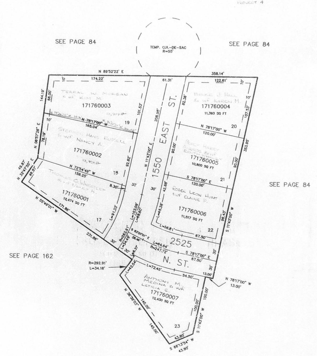
7' UTILITY & DRAINAGE EASEMENTS EACH SIDE OF PROPERTY LINES AS INDICATED BY DASHED LINES EXCEPT AS OTHERWISE SHOWN.
